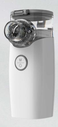
The device forms nebulizing effect by the following actions, the high-frequency vibration of piezoelectric ceramic piece leads to the deformation of micro plate, so that the liquid in contact with the micro plate is atomized. It is powered by a 5 V power adapter or a 3.7 V lithium battery, with the advantages of compact and portable design, easy to use, adjustable (two grades) and high in nebulization rate, which is applicable for use in hospital, clinic and family.
