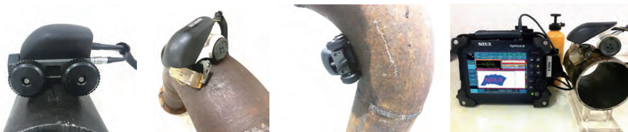
Corrosion mapping crawler
