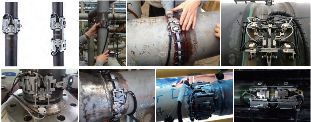
Phased array butt weld inspection crawler
