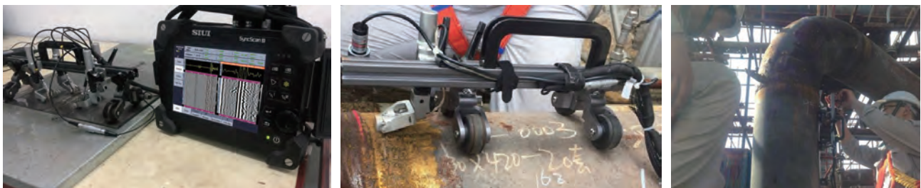
Phased array & TOFD crawler
